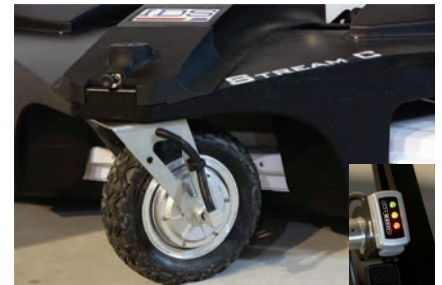
Stream C pivoting and motorized front wheel
