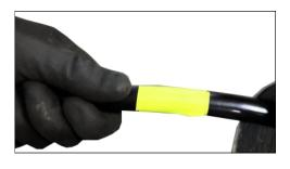
Attach a visual marker (tape) to the outer casing of the flexible shaft. Place it around half a metre from the end point of the shaft. The mark will indicate the chain's location and prevent possible injuries when the Pipe Cutter is removed from the pipe, including injury by rotating parts.
