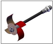
is also very effective for removing tree roots from the pipes. The front grinding discs are available in metal and plastic forms. Metal panel is more aggressive compared to the plastic panel. The diameter of the grinding discs is dependent on whether it is being used in a lined or unlined pipes (DN100 (4") and DN150 (6") pipe sizes). The smaller size plate should only be used in lined pipes.
